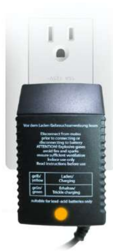
Yellow indicates charging
